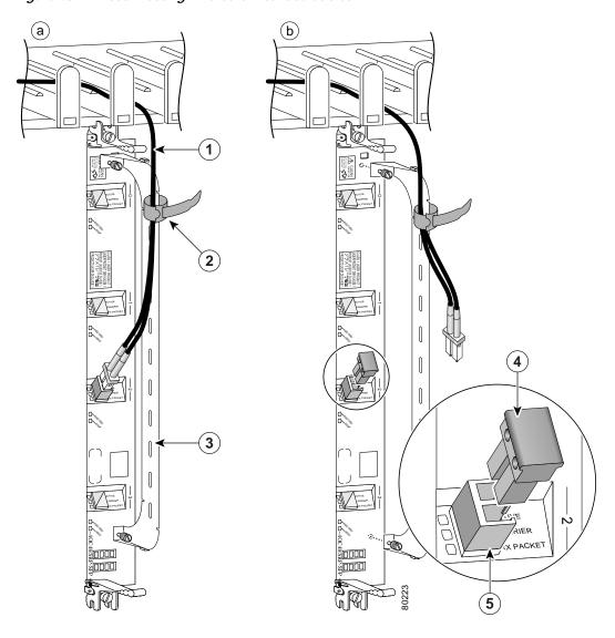
Figure 40 Disconnecting Line Card Interface Cables
